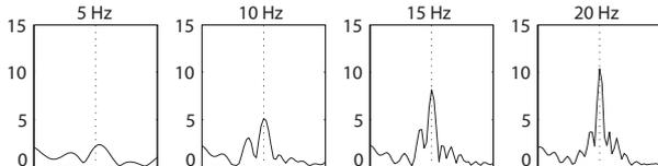
Figure 7: The effects of using different *cutoff frequencies* when extracting acceleration of a *hand clap*. The collision is more easily detected if the cutoff frequency is above 10 Hz (acceleration in  $\text{m/s}^2$ ).
