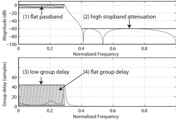
**Figure 2: The frequency domain plot of an IIR low-pass filter. The filter objectives are highlighted.**
