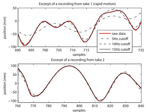
**Figure 6: Excerpts from Take 1 and Take 2. While a 5 Hz filter cutoff works well for the Take 2 below, the rapid motion needs a 10 Hz or a 15 Hz cutoff frequency to follow the details in the recording.**
