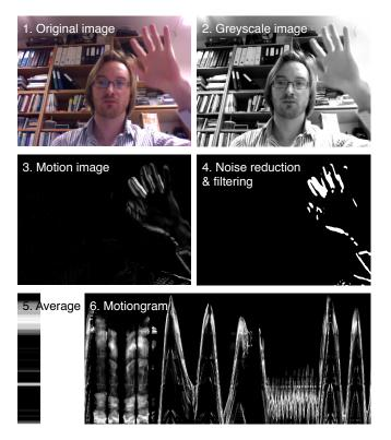
Figure 1. The steps involved in creating a motiongram: greyscale conversion (2), frame differencing (3), filtering (4), averaging (5) and plotting over time (6).
