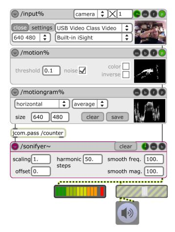
Figure 4. From the help patch of the **jmod.sonifyer** $\sim$  module. The video input module is connected to a module creating the motion image and then to the motiongram module. Finally, the output motiongram is sent to the sonifyer module for the creation of sound.
