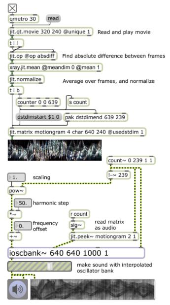
Figure 3. A minimal Max implementation for generating the sonification from video input. The oscillators are created in the **ioscbank** $\sim$  object, and Jitter matrix data is converted to an audio signal with the **jit.peek** $\sim$  object.
