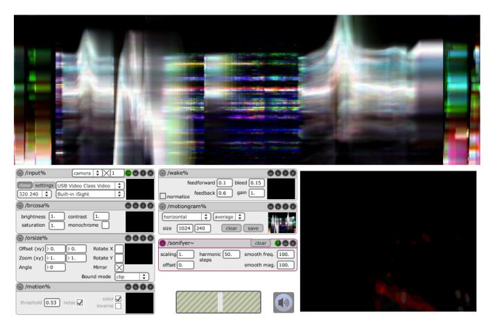
Figure 5. Performance patch using various types of video effects to modify the motiongram, and hence the output sound. The visual result from changing various video parameters can be seen in the motiongram at the top.
